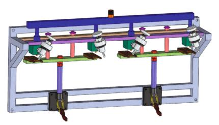
About 20-24 bottles (of size 300 ml) can be filled per minute depending on the speed of the operator. To make soft drinks, the bottles are prefilled with the required quantity of syrup flavor and then soda is filled. The soda and syrup mix inside the bottles to make soft drink.
