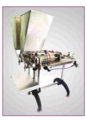
Filling is initiated with the help of an electrically operated foot switch. The table holding the bottle / container to be filled can be adjusted as required. The machine can be set to dose automatically also according to the efficiency of the operator. Depending on the quantity per fill, the viscosity and type of liquid/paste, the machine can fill about 6-10 bottles/containers per minute.
