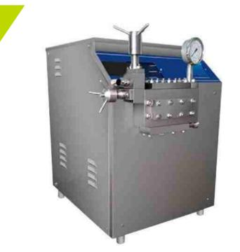
The machine is sturdily built and all contact parts are SS 304. It is available with the following output capacities
