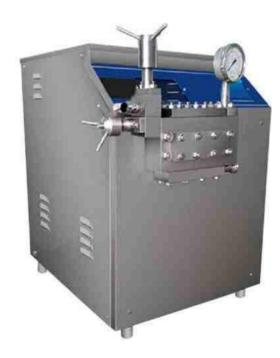
The machine is sturdily built and all contact parts are SS 304. It is available with the following output capacities
